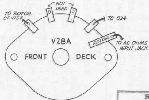
WIRING VIEW OF ALL DECKS OF SWITCH V28 VIEWED FROM REAR OF CABINET. BOTTOM OF CABINET IS AT TOP OF EACH DECK (They may be mounted either way however) . . . .
