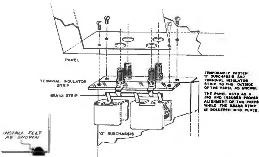
**Note:** After the tuning condensers are mounted on the "Q" sub-chassis, mount the insulated terminal strip and the sub-chassis temporarily upside down on the panel. The panel now acts as a jig and the connections between the condensers and the terminals can readily be made.
