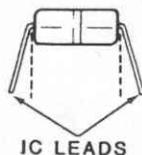
2. Before you install the IC, lay it down on its side as shown below and very carefully roll it toward the pins to bend the lower pins into line. Then turn the IC over and bend the pins on the other side in the same manner.
