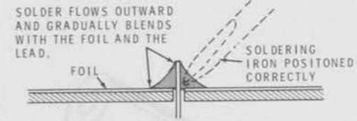
When you heat the lead and the circuit board foil at the same time, the solder will flow evenly onto the lead and the foil. The solder will make a good electrical connection between the lead and the foil.
