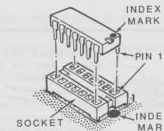
If it ever becomes necessary to remove an IC from its socket, insert the end of a screwdriver blade under the IC and gently move it up and down until the pins are free of the socket holes. Then carefully remove the IC.
