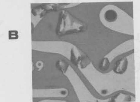
Use only enough solder to make a good connection, and lift the soldering iron straight up from the circuit board. If a solder bridge should develop, turn the circuit board foil-side-down and heat the solder between connections. The excess solder will run onto the tip of the soldering iron, and this will remove the solder bridge. NOTE: The foil side of most circuit boards has a coating on it called "solder resist." This is a protective insulation to help prevent solder bridges.
