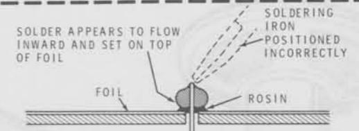
When the foil is not heated sufficiently the solder will blob on the circuit board as shown above. To correct, reheat the connection and, if necessary, apply a small amount of additional solder to obtain a good connection.
