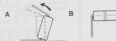
Before you install an IC, you must first identify the pin 1 end. Make sure this end of the IC is positioned over the index mark on the circuit board, as shown. Also make sure that all of the pins are started into the socket. **NOTE:** An IC pin can become bent under the IC and it will appear as though it is correctly installed in the socket.
