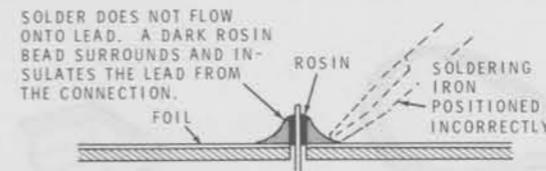
When the lead is not heated sufficiently, the solder will not flow onto the lead as shown above. To correct, reheat the connection and, if necessary, apply a small amount of additional solder to obtain a good connection.
