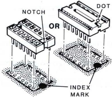
Hold the socket in place while you turn the board over and lay it on top of the socket on your work surface. The board will hold the socket in place. At first, solder only two pins at diagonally opposite corners of the socket. When the solder cools, check to make sure the socket is tight against the circuit board. If not, reheat the pins while you press against the socket to reseat it. Then solder the remaining pins to the foil.
