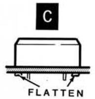
FLATTEN THE END POSTS WITH YOUR SOLDERING IRON TIP.
