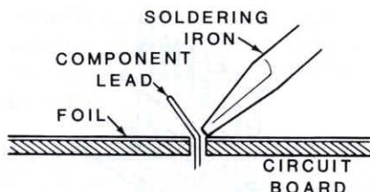
2. Apply solder to the other side of the connection. **IMPORTANT:** Let the heated lead and the circuit board foil melt the solder.
