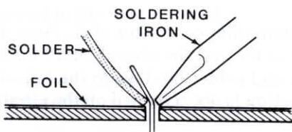
3. As the solder begins to melt, allow it to flow around the connection. Then remove the solder and the iron and let the connection cool.
