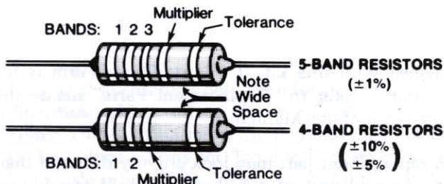
Occasionally, a "precision" or "power" resistor may have the value stamped on it. The letter R, K, or M may also be used at times to signify a decimal point, as in:  $2R2 = 2.2 \Omega$
