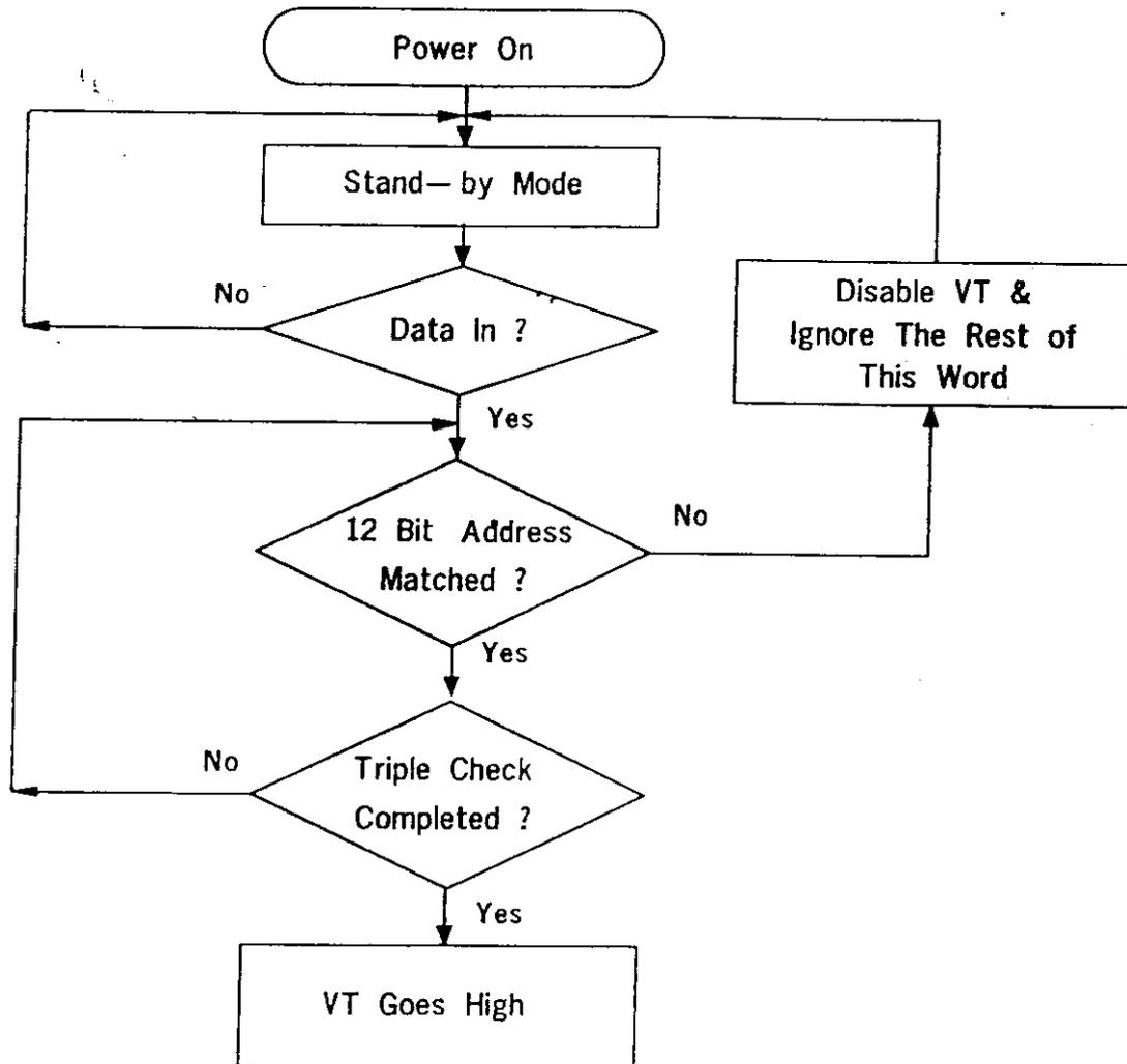
Note: The oscillator is disabled in stand-by state and activated as long as a logic 'high' signal applied to DIN pin. i.e. the DIN should be kept in logic 'low' during no signal input.
