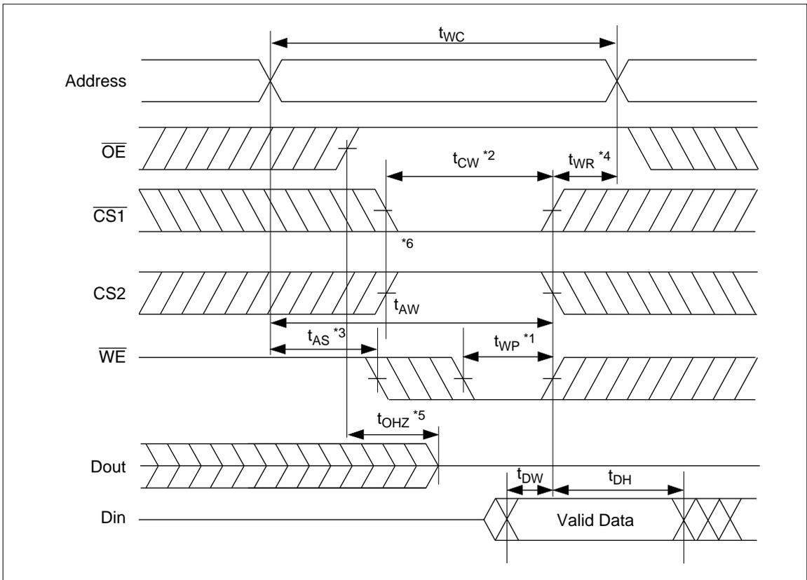
Write Timing Waveform (2) ( $\overline{OE}$  Low Fix)
