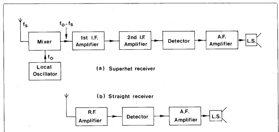
Figure 11. The superior complexity of the superhet against the simplicity of the straight receiver; both popular designs in the 1930's.
