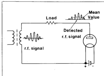
Figure 7. Detection of r.f. wave with diode valve.
