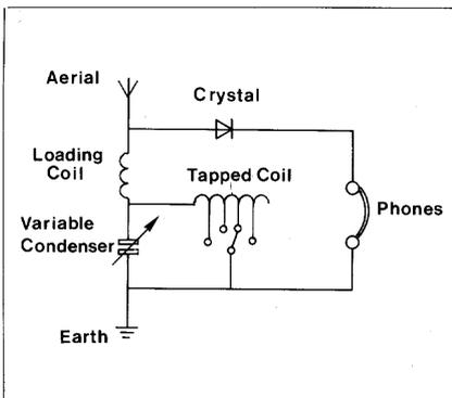
**Figure 10. Circuit of a typical 'tapped inductance' type of crystal set of the 1920's.**
