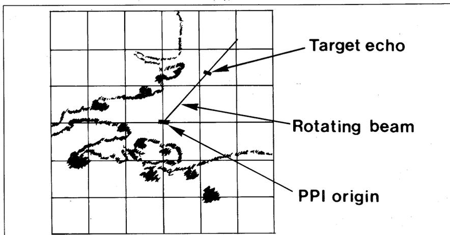
Figure 14. Typical return from PPI display. The rotating beam illuminates both the target and the main topographical features, e.g. coastline and towns. In this case the PPI equipment is on a ship in the Thames estuary.
