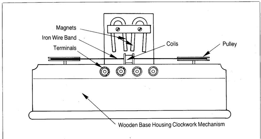
Figure 4. Simplified diagram of Marconi's magnetic detector (the Maggie).
