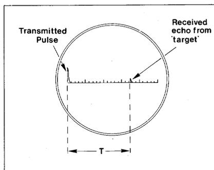
Figure 12. The basic principle of RADAR; the time  $T$ , the return journey time of the radio wave, is direct measure of the distance to the target.
