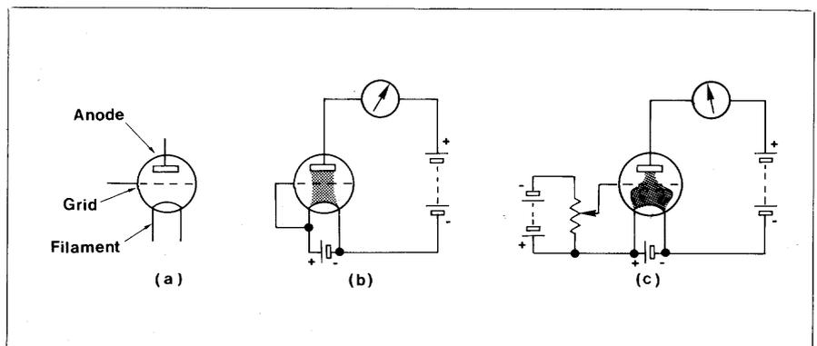
Figure 8. (a) The 'audion' or the first triode valve. (b) The grid has little effect when taken to filament potential. (c) Anode current is reduced when the grid is made negative with respect to the filament.
