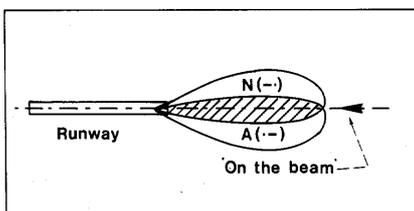
Figure 9. The Beam Homing System for Aircraft.
