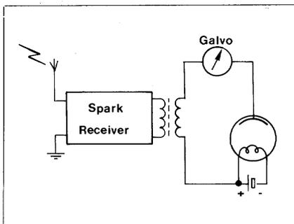
Figure 5. Fleming's arrangement for establishing the principle of the 'oscillation valve'.
