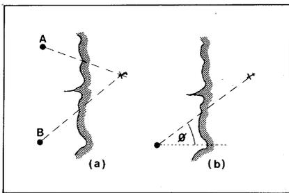
Figure 13. (a) The 'hostile' is located at the intersection of the beams from two stations, A and B. (b) A single station fixes both the range and bearing of the 'hostile'.
