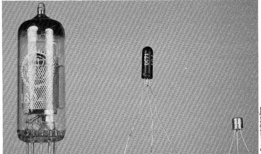
Thirty years of development:- a miniature valve of the 1950s compared with the once popular Mullard OC71 (a germanium PNP device) and the Ferranti ZN414, a complete AM radio in a TO18 can.
