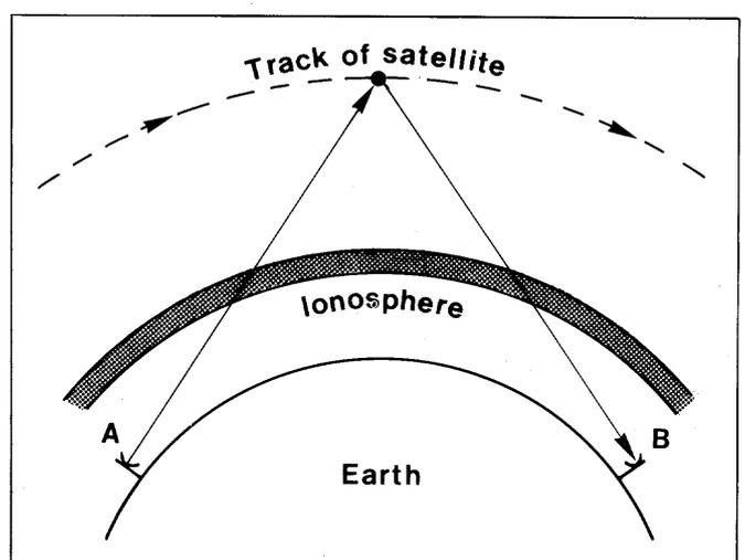
Figure 16. Effective 'line of sight' communication between two points, A and B, on the Earth's surface via orbiting satellite.
