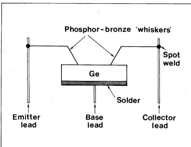
Figure 15. Construction of early point-contact transistor.
