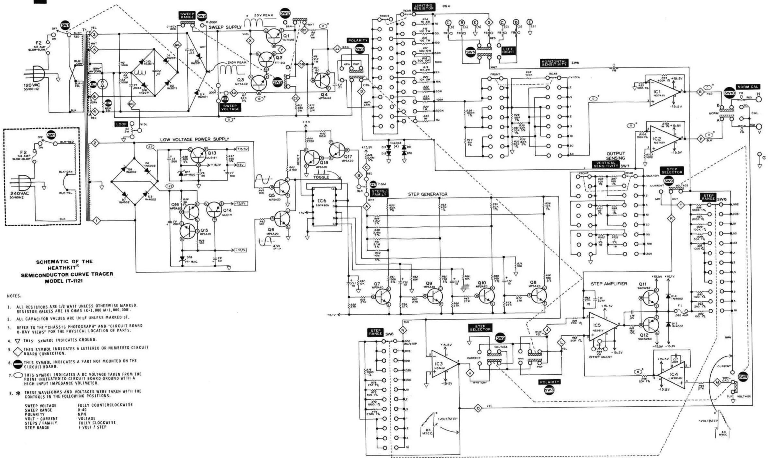
**SCHEMATIC OF THE HEATHKIT<sup>®</sup> SEMICONDUCTOR CURVE TRACER MODEL IT-1121**
