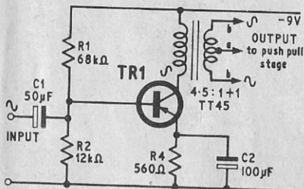
Common emitter stage with a collector current of about 3mA. The collector load is the transformer primary coupled to a class B push-pull pair. Special packages containing all three transistors (matched) can be obtained. If the characteristics are dissimilar, severe distortion is likely. Ideally the two halves of T1 secondary should be bifilar wound, i.e. both halves wound at the same time so that the wires lay side-by-side. Commercial types are available (e.g. Repanco TT45).
