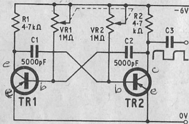
Free running square wave generator. Unbalance between two stages causes TR1 (or TR2) to conduct while TR2 (or TR1) is cut off. Cross-coupled capacitors C1 and C2 are alternately charged through base emitter junctions; discharged through VR1 and VR2. When C2 is discharged through VR2, TR1 base voltage falls exponentially to zero, when TR1 starts to conduct. TR2 is cut off. When C1 is discharged through VR1, TR2 base falls to zero, when TR2 will conduct. The small negative pips on the
