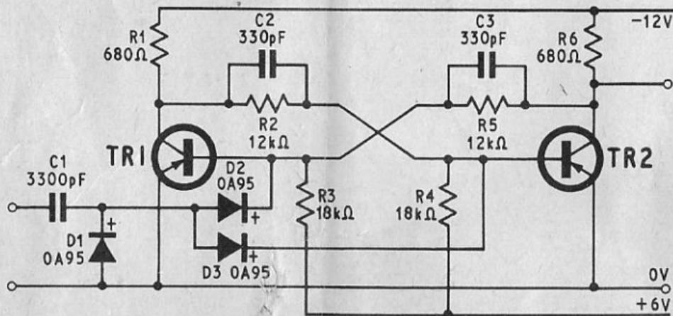
Commonly used for counting and generating square waves from pulse inputs.
