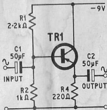
High input impedance; low output impedance. Often called an emitter follower. Decoupling capacitor is sometimes connected across supply lines to reduce power line impedance. Collector is common to input and output circuits. Used to match amplifier to low impedance load. Phase shift zero; a.c. current gain high; a.c. voltage gain  $< 1$ .
