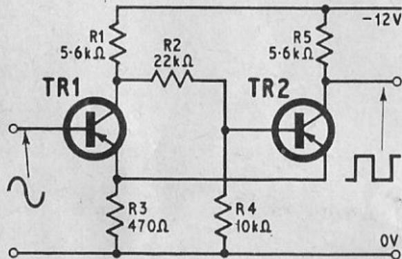
The Schmitt or emitter coupled bistable, can be considered as a fast acting switch, the action of which is precipitated by a pre-arranged d.c. level, the trip voltage (see waveforms). Often employed as a voltage level detector.
