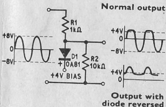
The shunt diode clipper uses the diode to short-circuit the output above the 4V bias. When the input voltage is less than the bias potential the output waveform is almost identical since the diode is not conducting. When the input voltage exceeds the bias potential the diode conducts and shunts the load resistance so that the output voltage only slightly exceeds the bias potential. With the diode reversed, the peaks are clipped at the bias voltage.
