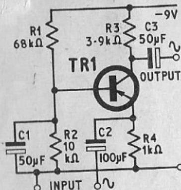
Low input impedance to emitter; high output impedance from collector. C1 acts as short circuit to a.c. while blocking d.c. Therefore, the base is grounded to a.c. and common to both input and output signal circuits. Used for matching low impedance source to amplifier stages. Phase shift zero; a.c. current gain  $< 1$ ; a.c. voltage gain high.
