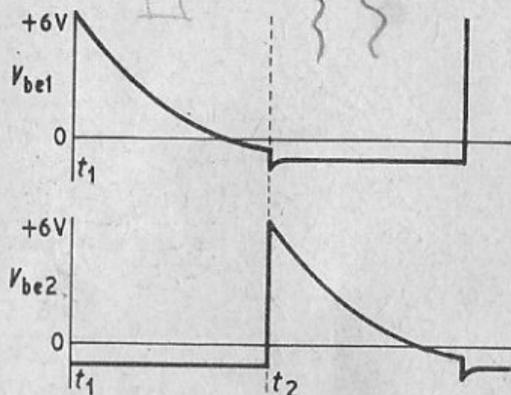
base waveforms are due to rapid initial recharge of capacitors. Waveform at both collectors approximate to a square wave. Frequency is adjusted by VR1 and VR2.  $f = 1/(1.4CR)$  where C is single coupling capacitance (farads) and R is base bias resistance (ohms), and where  $C1 = C2$  and  $VR1 = VR2$ . Mark/space ratio is altered by varying the value of one capacitor.
