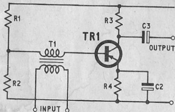
Low input impedance; source can be coupled in series with base instead of in the emitter circuit, where high current gain is required and where the normal common base circuit is unsuitable. Transformer can be used to match almost any impedance to the base. A.C. signal is superimposed on very small base bias current, determined by values of R1 and R2. Values of components not given because they depend on the characteristics of the transformer and signal source impedance.
