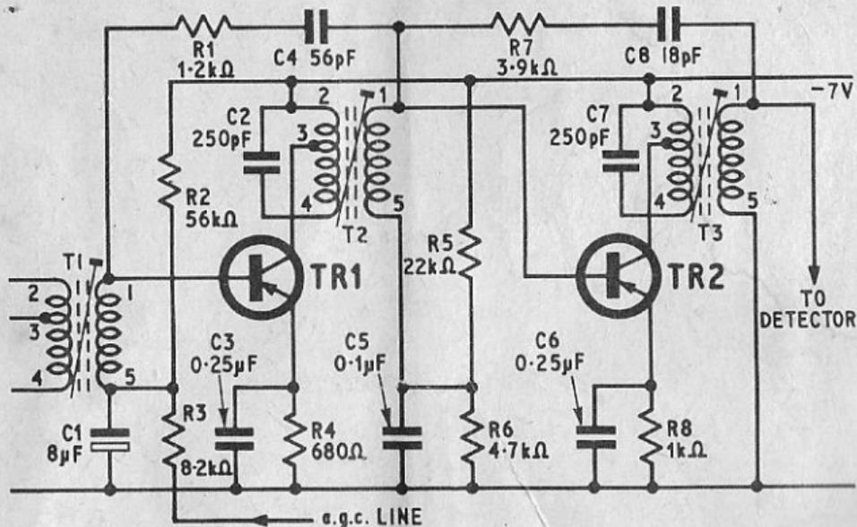
Tuned amplifier with transformer primaries tuned to the i.f. High frequency transistors essential. Base voltage is determined by potential divider (R2 and R3) in conjunction with a.g.c. voltage. Base of TR1 is current driven by T1; primary is connected to the r.f. mixer (not shown). Second
