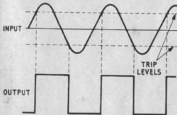
emitter drop at TR1) this transistor begins to switch on and TR2 switches off. Since there are no coupling capacitors in this circuit, reversion to its original condition of TR2 on can only be achieved by reducing the amplitude of the input signal below the trip voltage. The switch on and switch off voltages differ in level and this property is often used to square, or clip, waveshapes.
