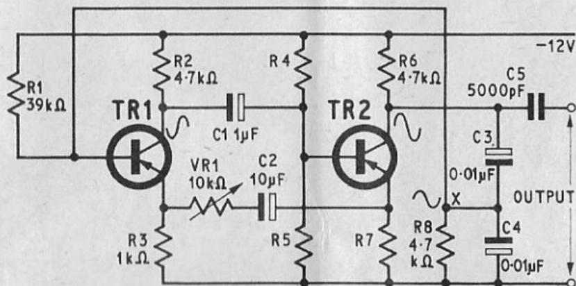
Audio frequency sine wave generator. Frequency determining components are contained in bridge network R6, C3, R8, and C4. Regenerative positive feedback from point "X" to TR1 base occurs only at this frequency. Frequency =  $1/(2\pi RC)$ . Here  $R = 4.7k\Omega$  and  $C = 0.01\mu F$ . Oscillator is frequency selective. Any change or mismatch in component values in the series
