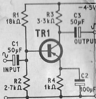
Medium input impedance. Medium output impedance. Battery positive supply line is common to both input and output circuits. Decoupling capacitor C2 short circuits emitter to positive supply line as far as a.c. is concerned. Therefore, emitter is common to both input and output circuits. Phase shift  $180^\circ$ ; a.c. current gain high; a.c. voltage gain high.
