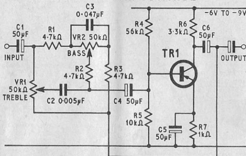
With any form of tone control the signal level will be reduced at pre-determined frequencies. If bass boost is required, the high frequencies are cut. Then the audio spectrum is amplified to bring them up to normal, while the bass frequencies will be higher than the treble. Similarly for treble boost the bass frequencies are cut. The reactance of a capacitor ( $X_C$ ) is inversely proportional to frequency. When the
