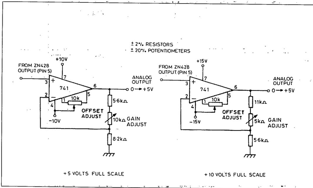
Fig.8 Unipolar operation - component values
