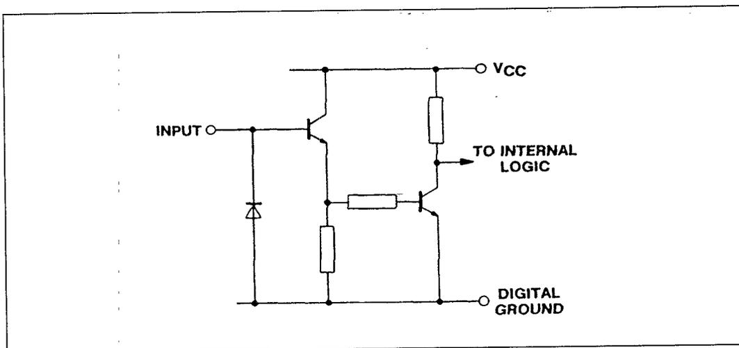
Fig.6 Equivalent circuit of all inputs
