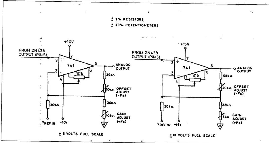
Fig.10 Bipolar operation - component values
