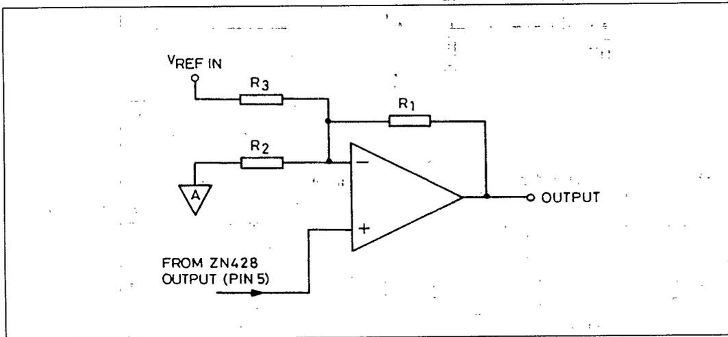
Fig.9 Bipolar operation - basic circuit
