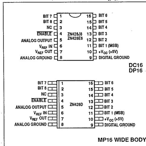
Fig. 1 Pin connections (not to scale) - top view
