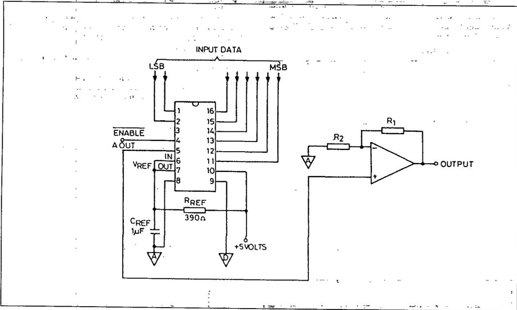
Fig.7 Unipolar operation - basic circuit
