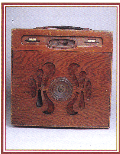
The 1929 Marconiphone Model 55 receiver mentioned in the text, pictured after a quick dusting down following its retrieval from the farmhouse loft. This 5-valve medium and long-wave battery set cost 18 guineas (£18.90) new, and was the first to be sold with an instruction booklet providing a list of spare parts, presumably to encourage owners to do minor repairs for themselves.
