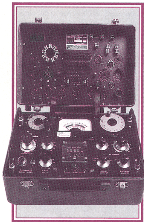
A versatile valve tester, the 'Test Set, Electronic Valve CT-160', produced by AVO for the Ministry of Defence, and now widely available on the surplus market.
